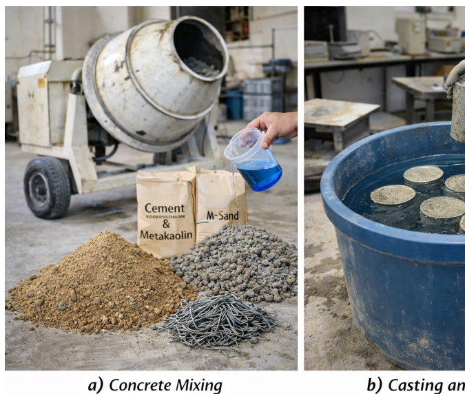
Fig. 2. Specimen preparation and curing: (a) concrete mixing, (b) casting and water curing.
