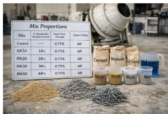
Fig. 1. Mix proportions and material constituents for different metakaolin replacement levels.
