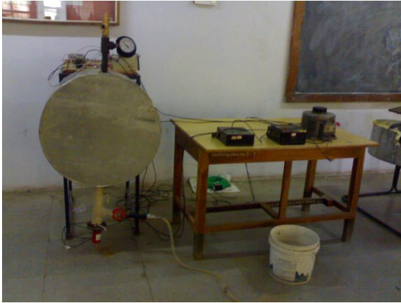
Fig. 6. Measurement of Conduction Heat Loss from the Receiver
