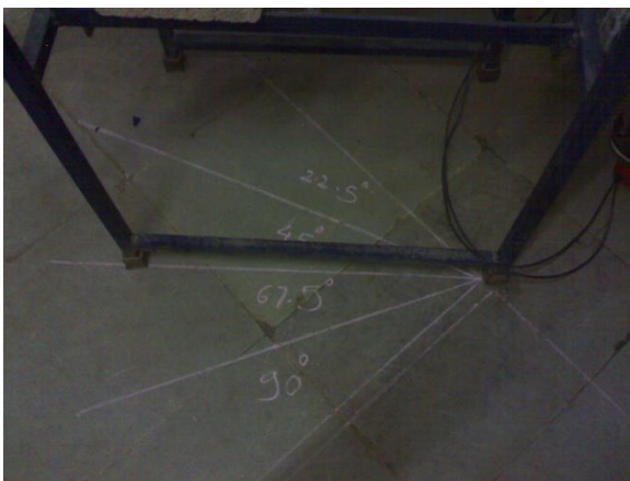
Fig. 7. Photograph for Angular Settings of the Receiver with respect to wind direction
