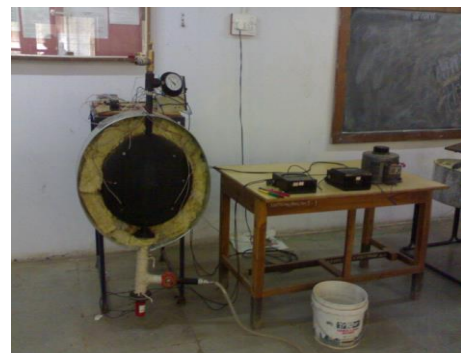
Fig. 4. Laboratory Arrangements for Heat Loss Measurement from the Receiver
