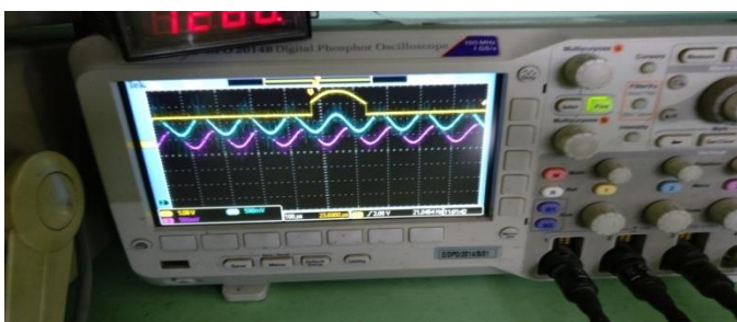
Fig05: Output signal of reflective encoder
