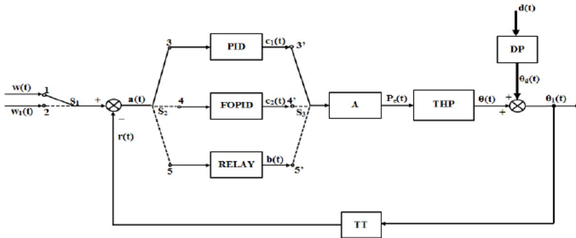
Fig. 4. Proposed temperature control structure for thermal (annealing) process using integer and fractional order PID schemes [4]
