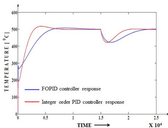
Fig. 5. The comparative graph between the control system step responses, for integer order PID and FOPID controllers [4]
