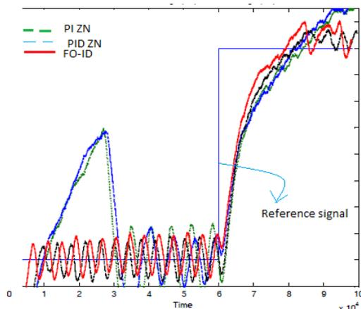
Fig.1. Comparison of output graphs between PI, PID, FO-ID, FO-PI controllers with the reference signal [3]
