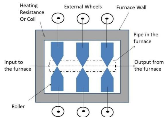
Fig. 2. The longitudinal section of the furnace which contains the centres of the external wheels [4]
