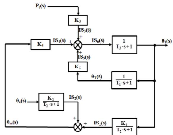
Fig. 3. Final Laplace domain structure of the thermal annealing process obtained through energy balance equation [4]
