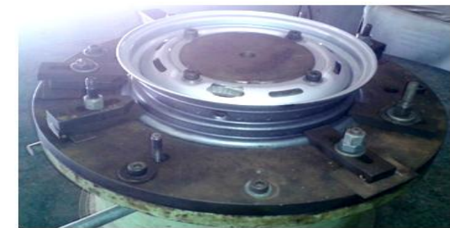
Fig 2. Dynamic cornering fatigue test set up.
