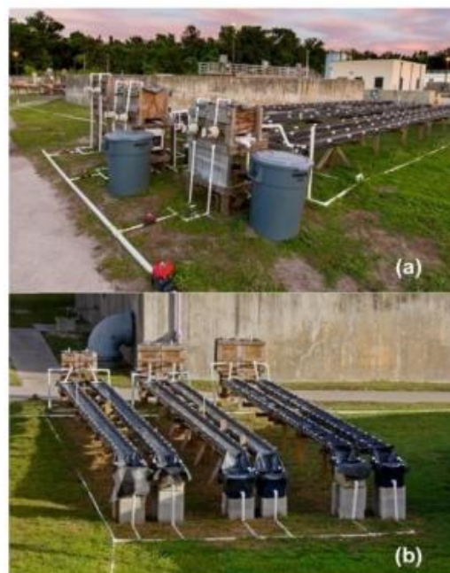
Fig. 3. Moss scrubber design with (a) inflow piping, tanks, and flow meters and (b) all six raceways with outflow filters. [7]
