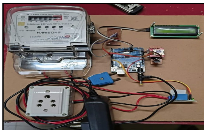
Fig. 1. GSM-Blockchain Based Energy Billing and Load Management system
