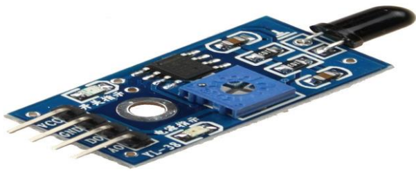
Figure(4): Fire sensor
